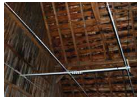
PHOTO 2: W1GN's full sized three-element single band Hygain LJ-153BA indoor Yagi.
